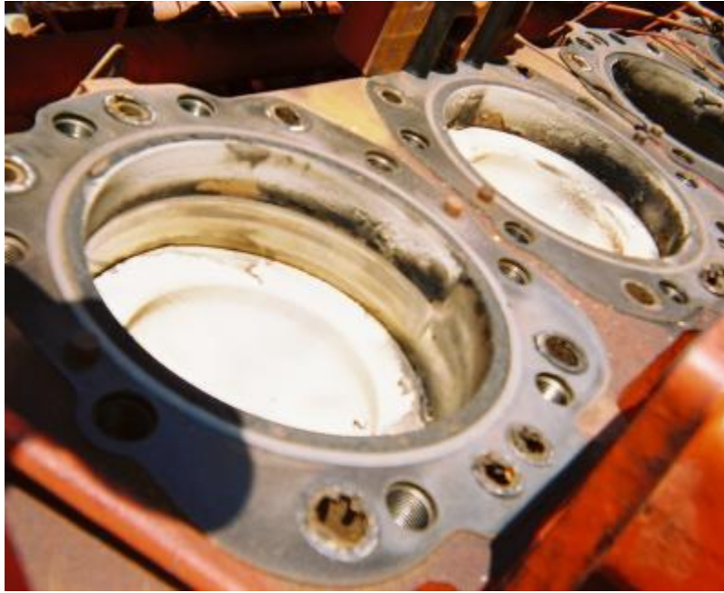
Figure 3. Siloxane Damage to Engine Pistons
